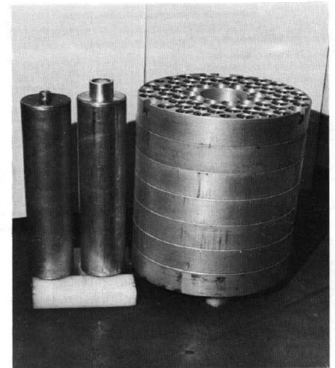
Fig. 1. The new aluminium matrix for the SEG-6 assembly in the RRR zero power reactor at the CINR
