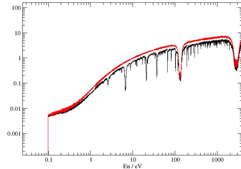
Preliminary transmission spectra for a pellet containing UO<sub>2</sub>+Gd grain
