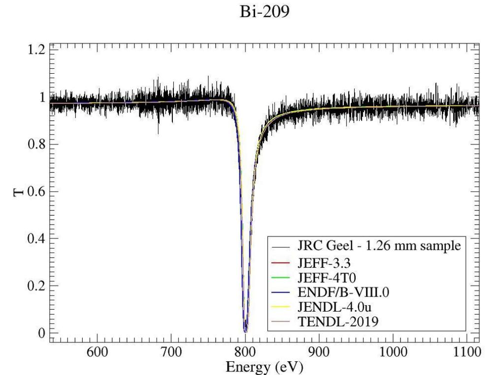
Comparison of experimental transmission for 1.26 mm sample with state-of-the-art nuclear data libraries at  $^{209}\text{Bi}$  first resonance (802 eV).
