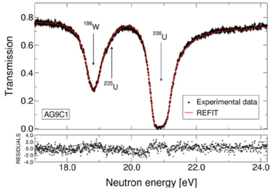
NRTA for a pellet containing UO<sub>2</sub>+Ag, showing a significant amount of W not reported in the specifications
