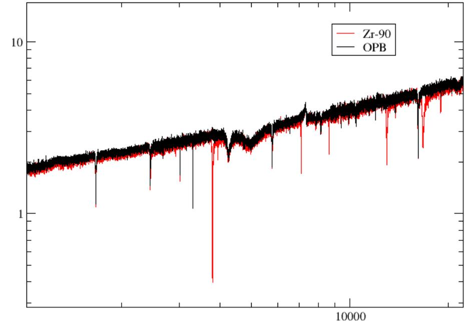
Preliminary TOF spectra for  $^{90}\text{Zr}$  transmission experiment
