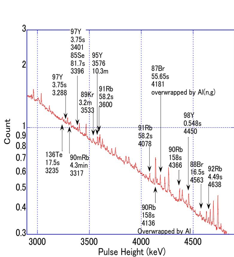
Fig. 5 Measured gamma-ray spectrum for critical core
