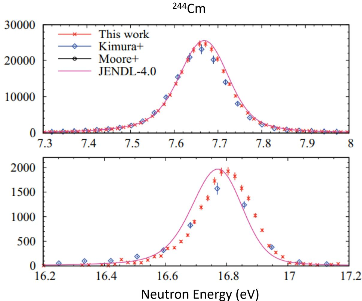
Neutron capture cross sections of  $^{244}\text{Cm}$  and  $^{246}\text{Cm}$  were (re-)measured in the energy range of 1 to 1000 eV with “Single-bunch mode”.
