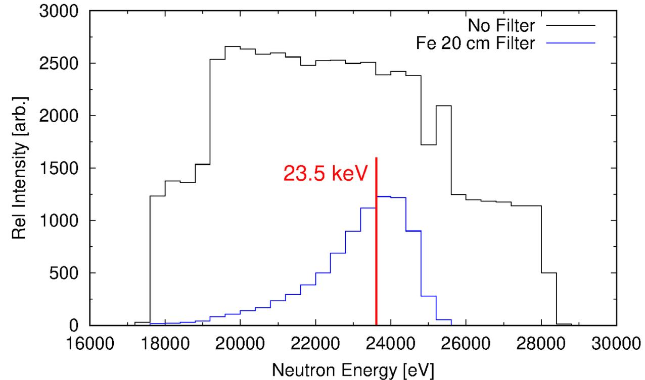
Energy distribution of the filtered neutron beam (blue) and its energy centroid (red) compared to the energy distribution without filter (black)
