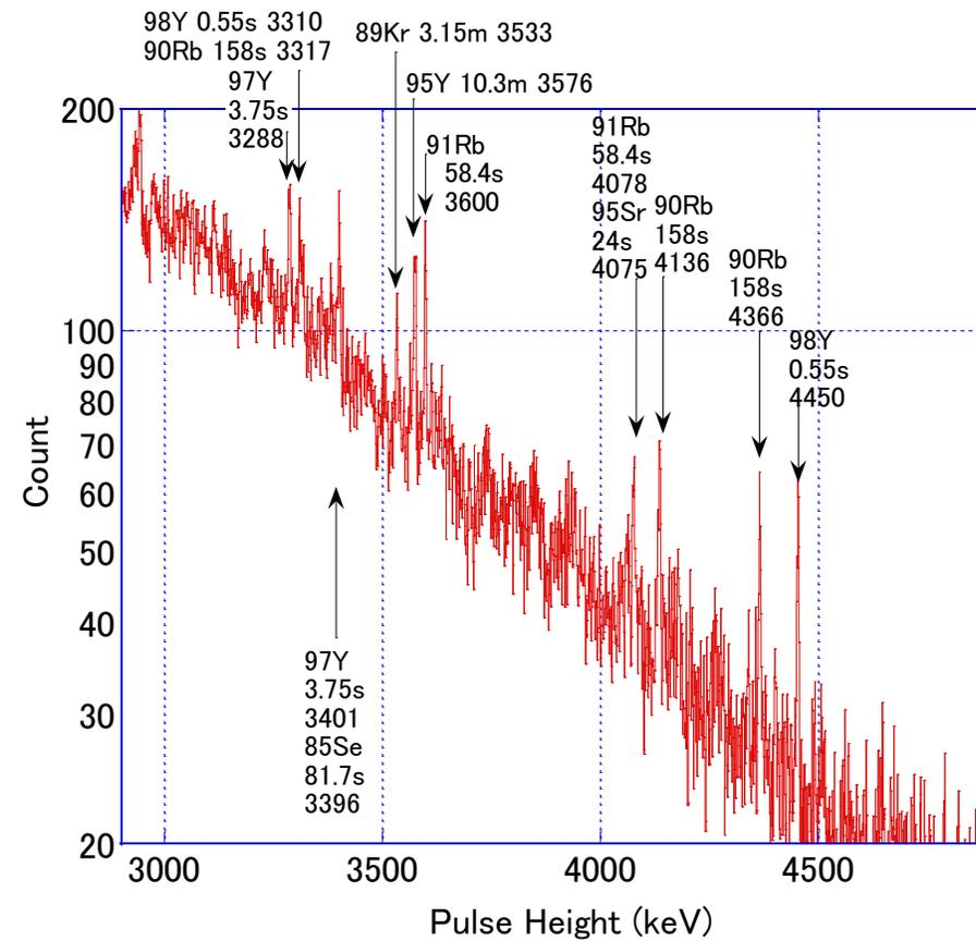
Fig. 6 Measured gamma-ray spectrum corresponding to the background TOF region in the experiment of KURNS-LINAC
