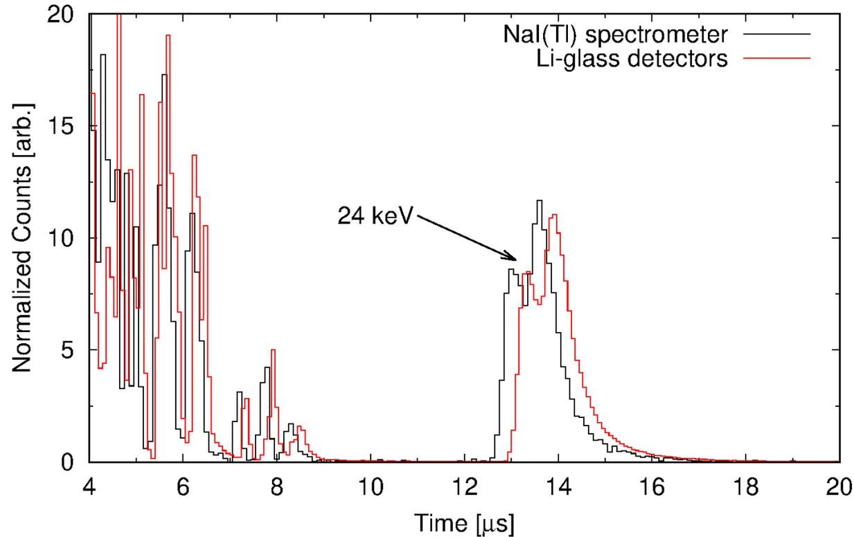
Filtered neutron beam through 20 cm of Fe measured by Li-glass detectors and a NaI(Tl) spectrometer (with B sample).
