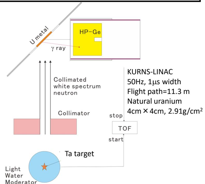
Fig. 4 experimental set-up of KURNS-LINAC
