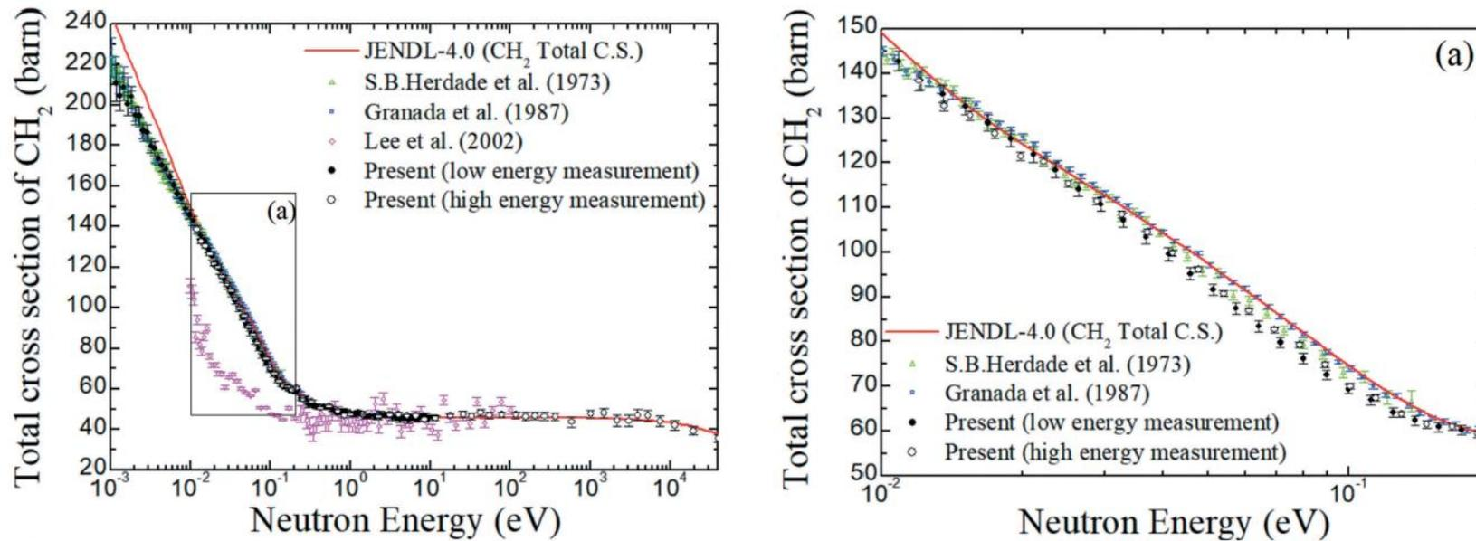
Fig. 7 Comparison of the present results with the previous measured results and the evaluated data for the neutron total cross sections of  $\text{CH}_2$
