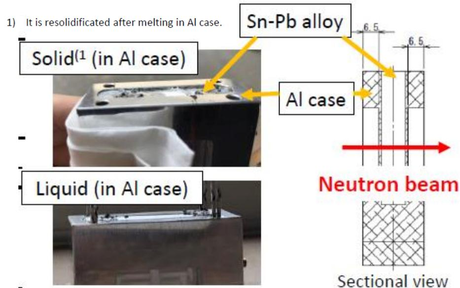
Fig. 1 Sn-Pb alloy sample
