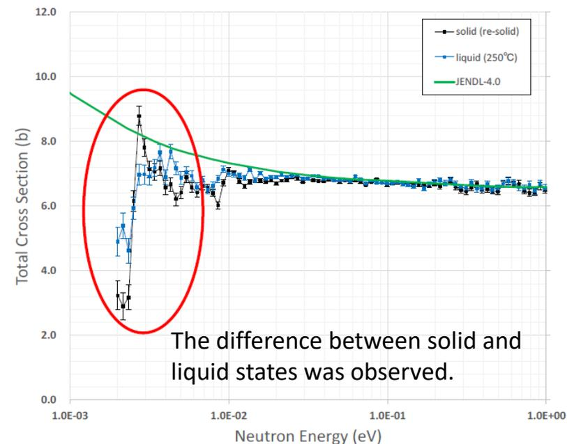
Fig. 2 Comparison of the total cross sections of Sn-Pb alloy in the solid, the liquid and JENDL-4.0 (free-gas model).
