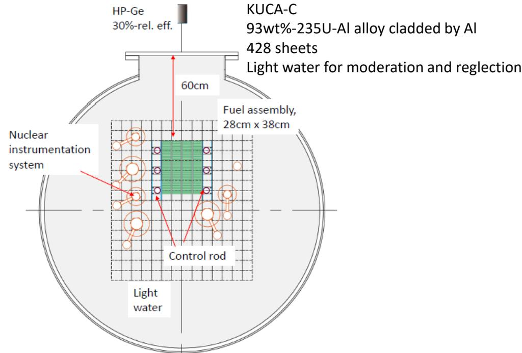
Fig. 3 experimental set-up of KUCA
