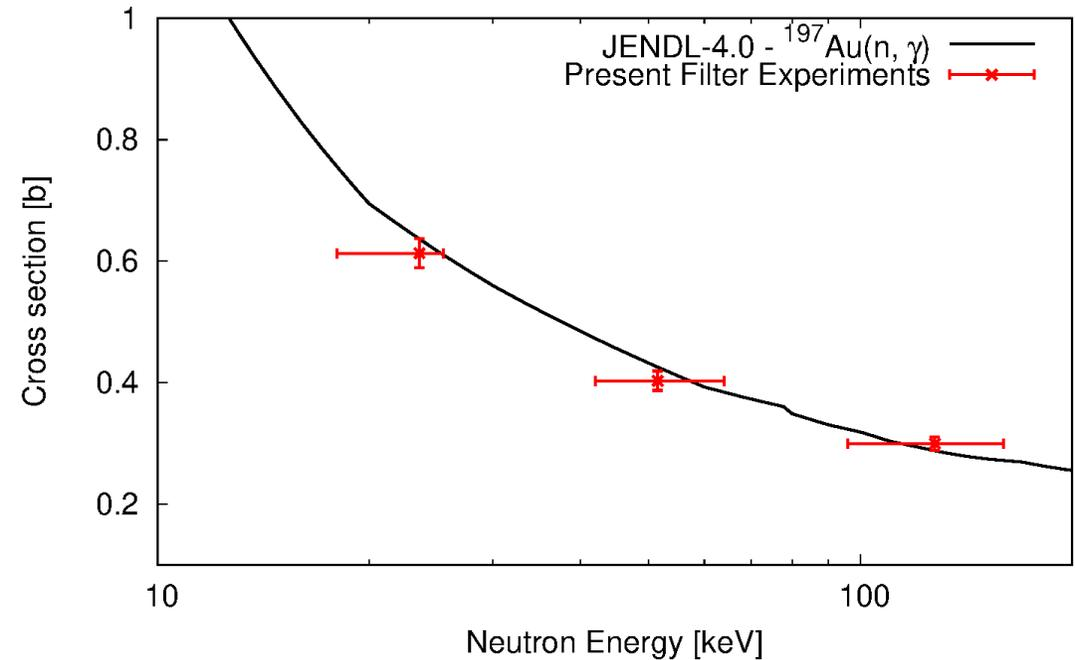
Cross-section results for the  $^{197}\text{Au}(n,\gamma)$  reaction using the neutron filters compared to the evaluated data from JENDL-4.0
