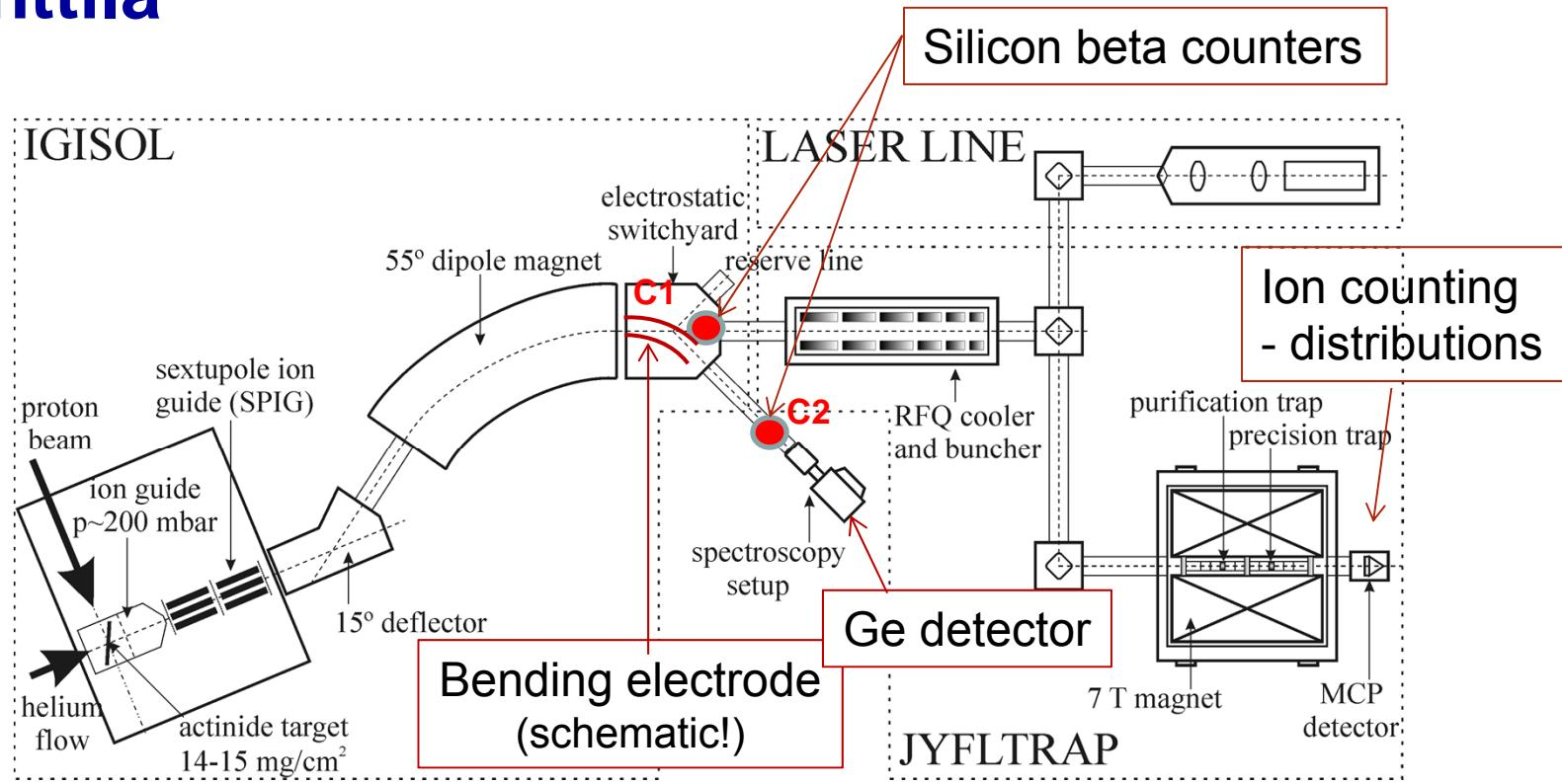
Fission yield to the spectroscopy line **1400 atoms/( $\mu$ C \* mbarn)**
