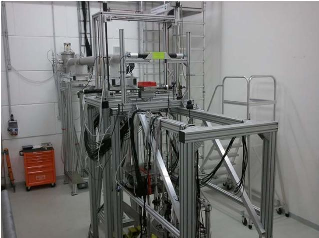
Transmission set-up for total cross sections
