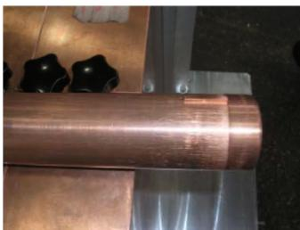
The block is made by Seven Cu plates (Oxygen Free) 60x60x10 cm<sup>3</sup> each (~ 2,25 tons total)
