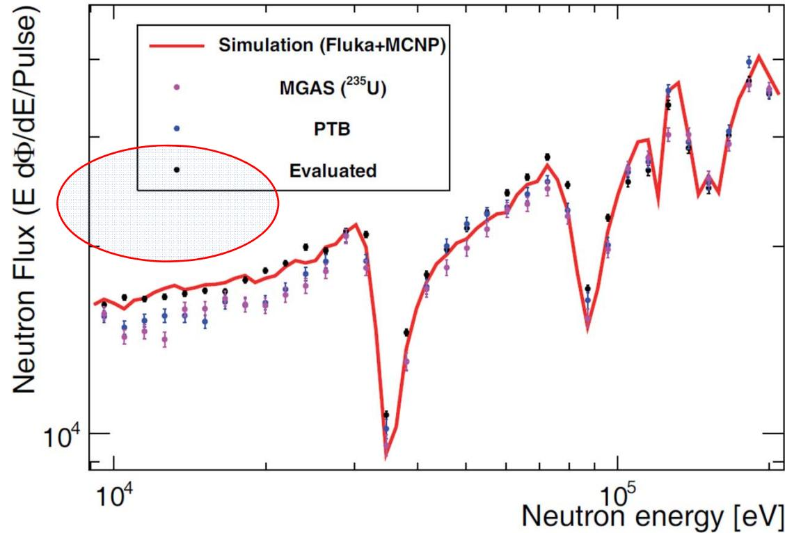
The **flux** calculated on the basis of the  $^{235}\text{U}(\text{n},\text{f})$  cross section **found systematically lower** than “expected” in the 10-30 keV range (*M. Barbagallo et al., Eur. Phys. J A 49 (2013) 156*).
