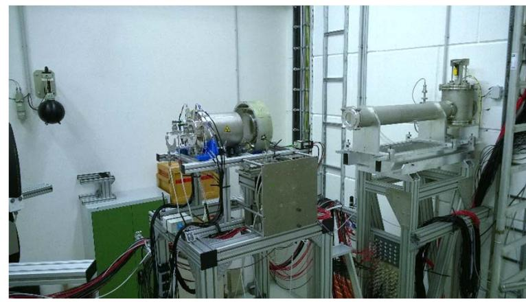
Neutron induced fission with two fission chambers
