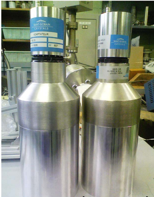
Gamma-ray detector, \text{LaBr}_3(\text{Ce}) Length = 5inch, Diameter = 4inch
