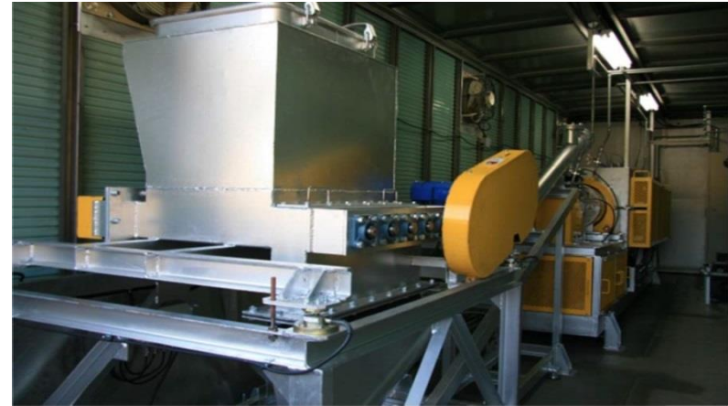
Incineration facilities for crop residues tested at a demonstration site in affected areas
