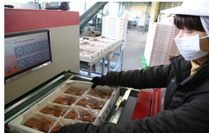
Anpo-kaki nondestructive inspection status (Yanagawa testing facility)
