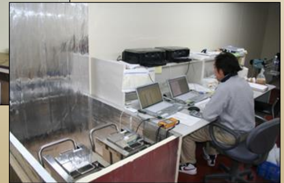
Measuring chamber to maintain constant temperature and humidity
