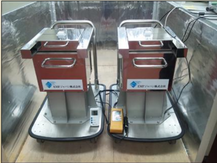
NaI scintillation gamma-ray measuring instrument (produced by EMF Japan)
