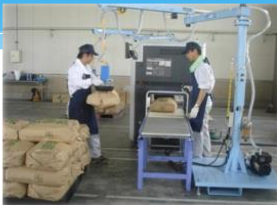
2. The bag is placed on a conveyor belt leading to the measurement device
