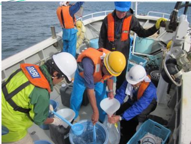
Distribution of seawater samples to NRA and IAEA containers after homogenization. The samples will subsequently be analyzed in parallel in Japan and the IAEA.
