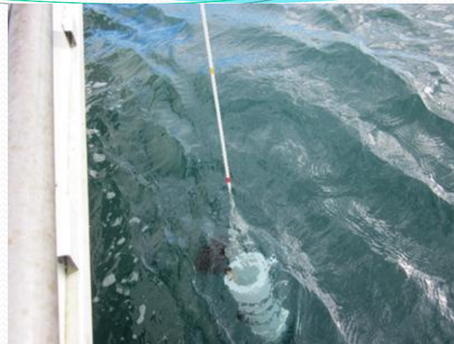
Collecting surface seawater during the mission using a Niskin bottle.
