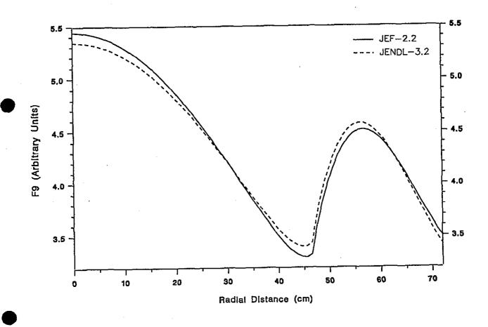
Figure 2: <sup>239</sup>Pu Fission Rate (F9) Radial Profiles, Axially Centered, Normalized to Equal Power, Obtained Using <sup>56</sup>Fe Data from JEF-2.2 and JENDL-3.2 in the Radial Reflector
