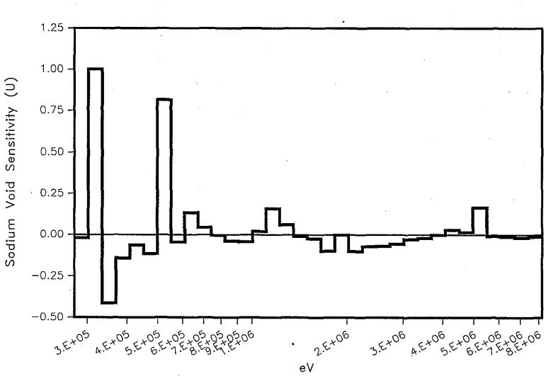
Figure 1: Energy Dependent Sensitivity Coefficient of the Sodium-Void Coefficient Due to the <sup>238</sup>U Inelastic Scattering Cross Section in the Fuel Region
