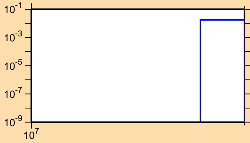
\sigma vs. E for ^{246}\text{Pu}(n,4n)
