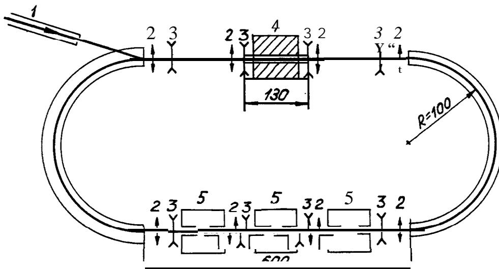
Fig. 1. Configuration of suggested demonstration facility. 1- deuteron linear accelerator; 2,3- magnet lenses; 4- target assembly; 5- RF resonators.
