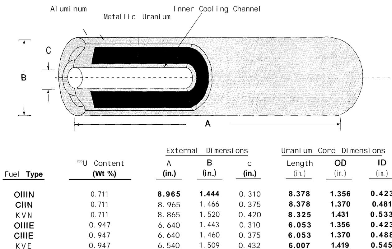
Figure 5. Typical Production Reactor Fuel Elements.
