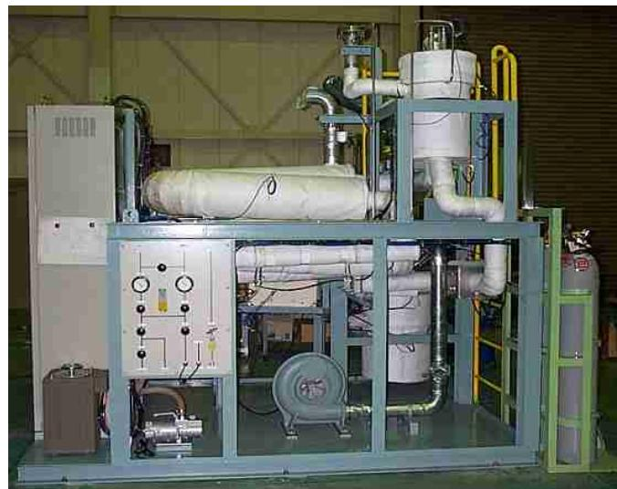
**Figure 12.3.16. Photo of CRIEPI static corrosion test facility**
