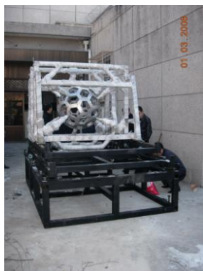
Fig.2 The external support and the honey comb
