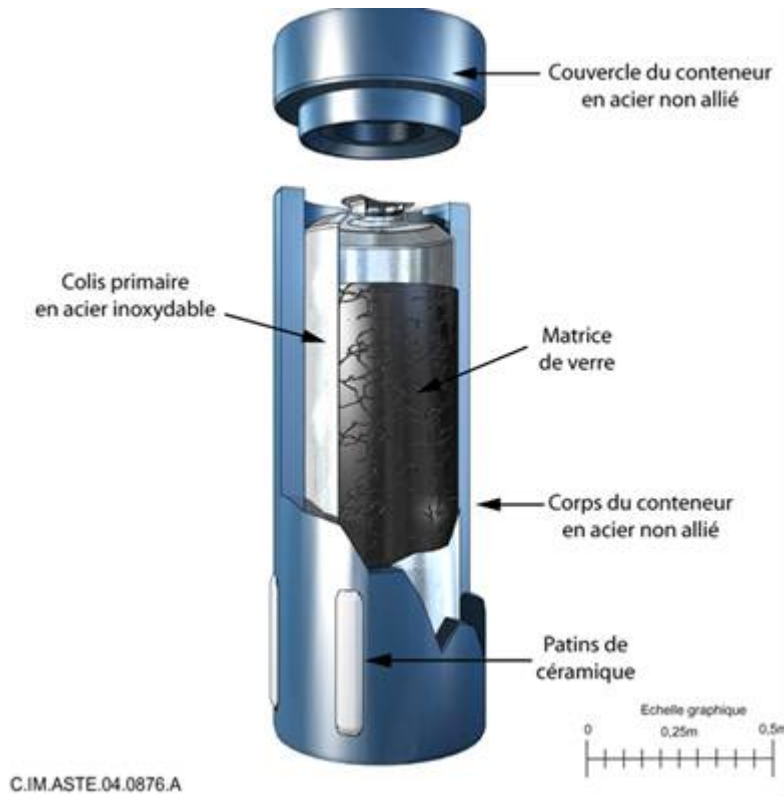
Schematic diagram of a disposal package for vitrified C reference packages (glass, container and overpack)
