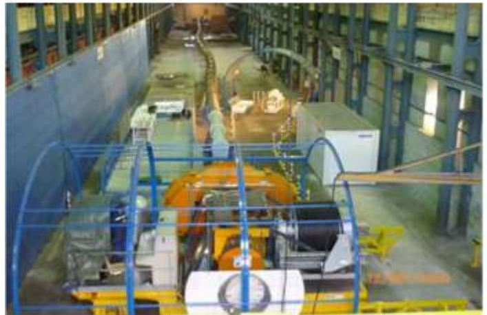
Fig. 3b: Retrieval of a disposal HLW package from a simulated emplacement cell in France (ESDRED programme, 2008)
