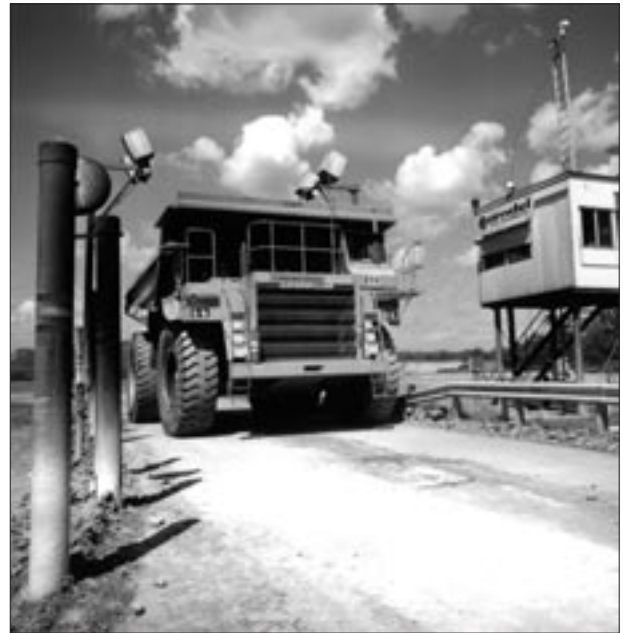
Determining ore grade with a radiometric discriminator at the Ranger Mine in Australia.
