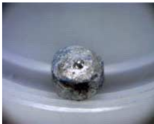
Figure 4. Cathode Cd ingot obtained after Pu electro-transport test at cathodic current density of 41 mA/cm 2
