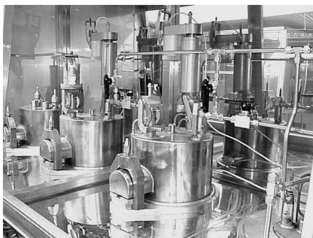
Fig. 1: Upper part of UF_6 , NpF_6 condensers with piping and measurement system
