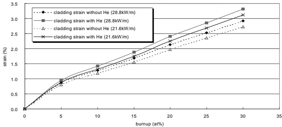
Figure 8. Cladding strain due to the clad thickness for the (U-TRU-Zr)-Zr dispersion fuel
