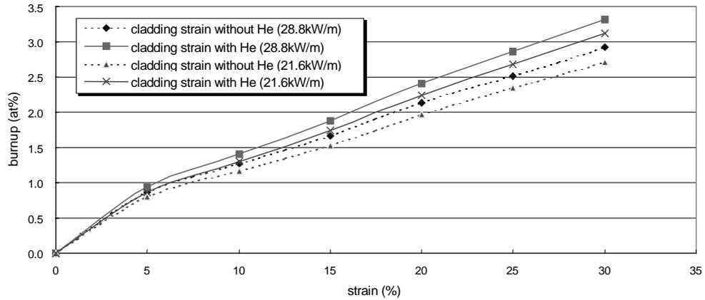
Figure 7. Cladding strain for the (TRU-Zr)-Zr dispersion fuel
