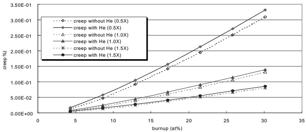
Figure 4. Cladding strain according to plenum-to-fuel ratio for the alloy fuel
