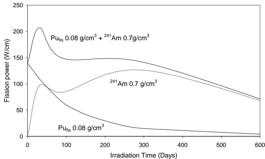
Figure 3 shows that <sup>241</sup>Am do not generate power at the start of the irradiation. The first maximum in the power generated in americium is due to fission of <sup>242m</sup>Am, while the second maximum is due to fission of <sup>239</sup>Pu. The power in the fissile plutonium decreases rapidly, while that in the americium remains relatively constant for a long period, reflecting the slow burn-up of the actinides present in the americium pin. From the computations can be concluded that:
