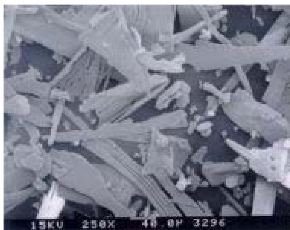
Figure 8. SEM photographs of ZrO_2 formed by pyrohydrolysis conclusion
