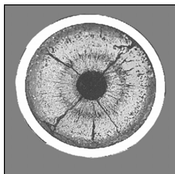
Figure 4. Macrostructure of irradiated fuel UNpO 2 (B=12.5%)
