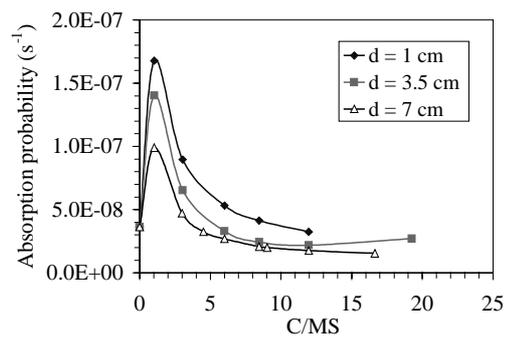
Figure 11. Absorption probability of  $^{244}\text{Cm}$
