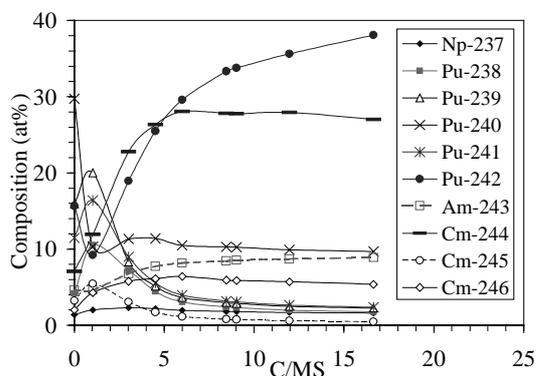
Figure 8.  $C/MS$  dependence of the equilibrium composition of individual actinides (atom%) in 7 cm channel
