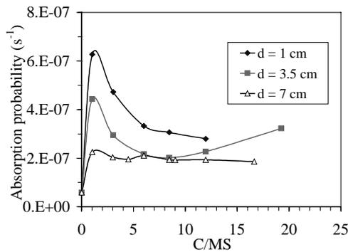
Figure 10. Absorption probability of  $^{242}\text{Pu}$
