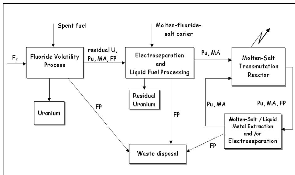
Experimental and theoretical studies in the field of **pyrochemical partitioning** technology development for the MSTR fuel cycle are oriented in particular to the following areas:
