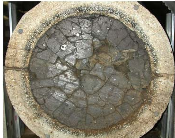
Crack Structure at Axial Midplane
