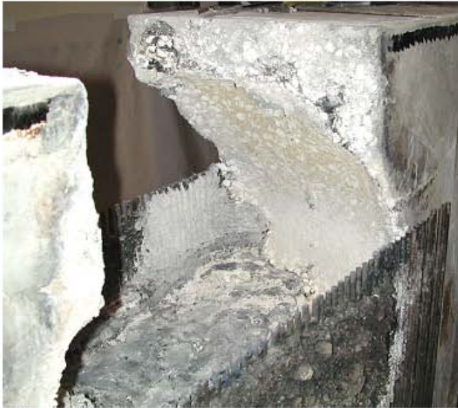
Corium and Concrete Walls
