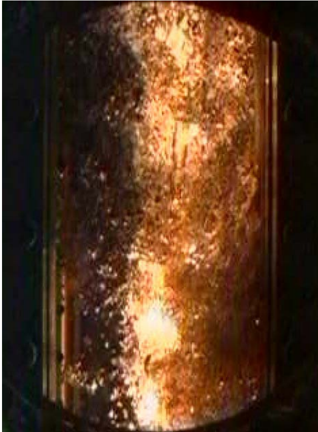
Corium melt mixing in KT-2 (CANON). Viewing area 10 by 20 cm
