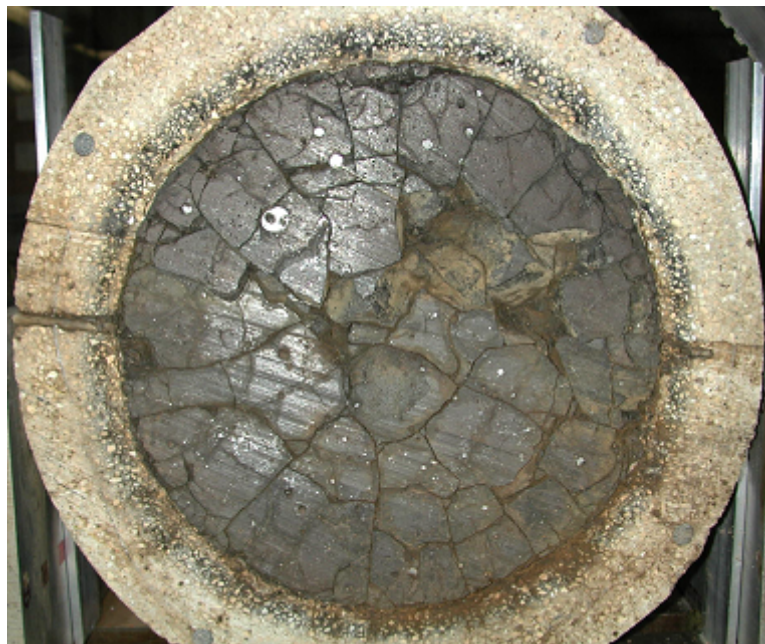
Figure 2. Extensive crack structure in the midplane sample of the SSWICS-3 crust
