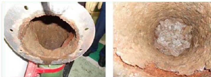
Figure 4.7: Photograph of the corrosion damage and clogging of the SNO overflow drainage pipe
