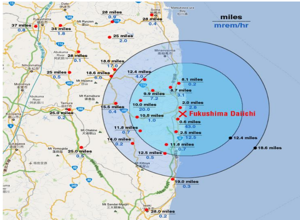
Figure 5.4-1 Initial Off-Site Survey Results
