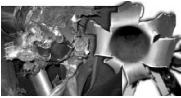
Hydrogen explosions in BWR piping have been identified as a recurring event.
