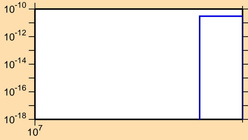
\sigma vs. E for ^{67}\text{Ga}(n,\text{pt})
